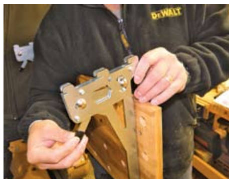
▲ The brackets adjust to two positions to sit horizontally or to tip back and retain a 90° position to the legs
